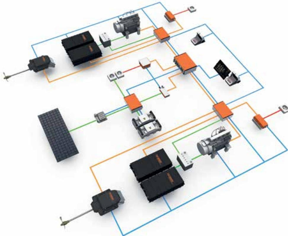
propulsion motor and a generator. The reduced electric propulsion, generator and battery demands of a parallel system reduce the costs compared to a serial system. Parallel systems are more likely to win initial market acceptance because of a perceived greater reliability, as the 'trusted' diesel engine is still connected to the propeller shaft with the electric propulsion adding a redundant system.
