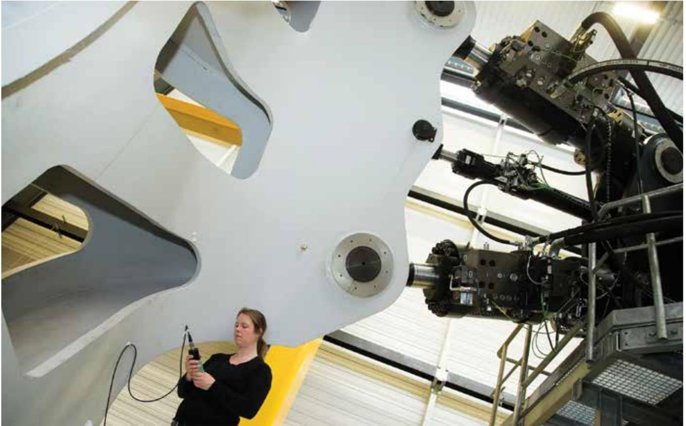
At the Dynamic Nacelle Test Rig, wind loads occurring in the field are emulated by servo-hydraulic actuators in a Stewart-platform configuration transmitting mechanical loading on rotor shaft of the specimen. Photographer: Martina Buchholz
