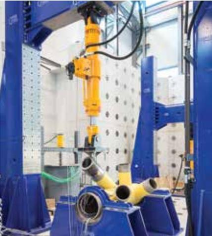
Examining the fatigue behaviour of large components under multi-axial loading. Photographer: Jan Meier
