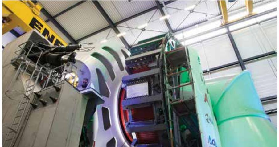
The comprehensive medium voltage grid emulator for electrical system testing covers all possible grid events and characteristics and helps shortening the certification process. Photographer: Martina Buchholz
