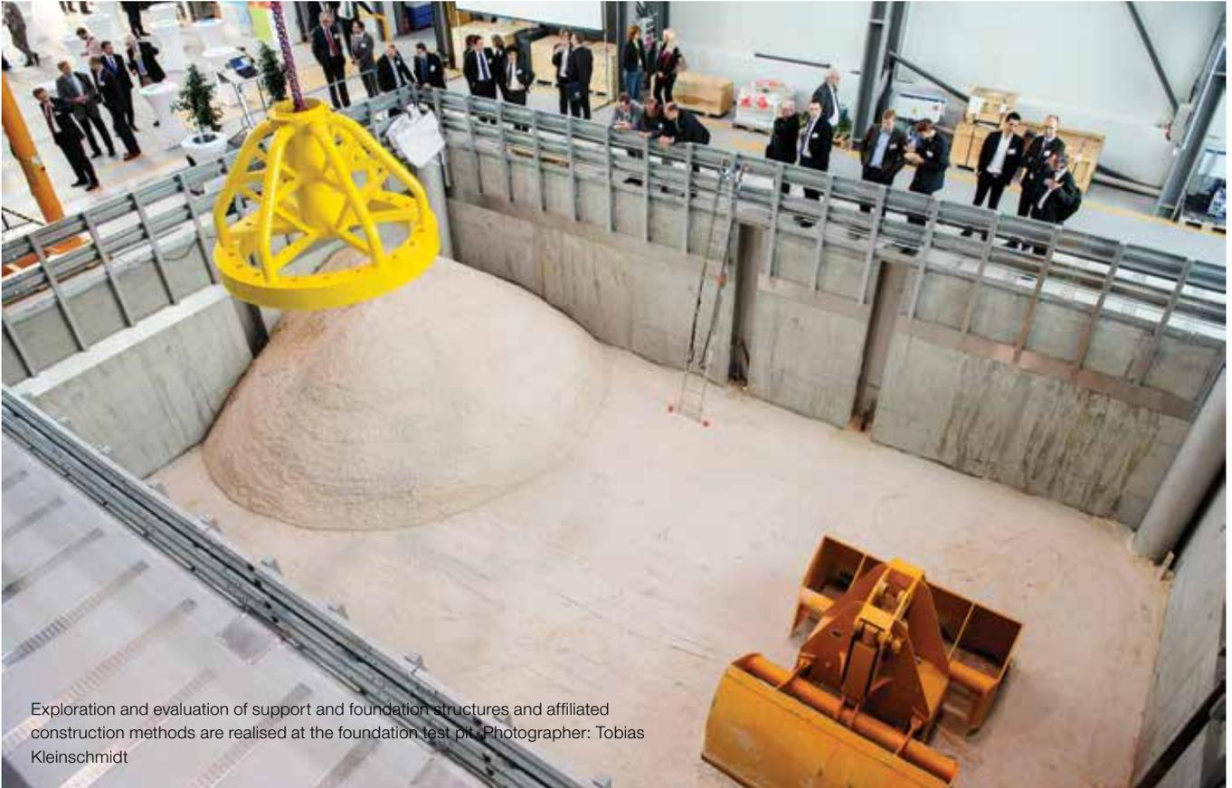
Exploration and evaluation of support and foundation structures and affiliated construction methods are realised at the foundation test pit. Photographer: Tobias Kleinschmidt
