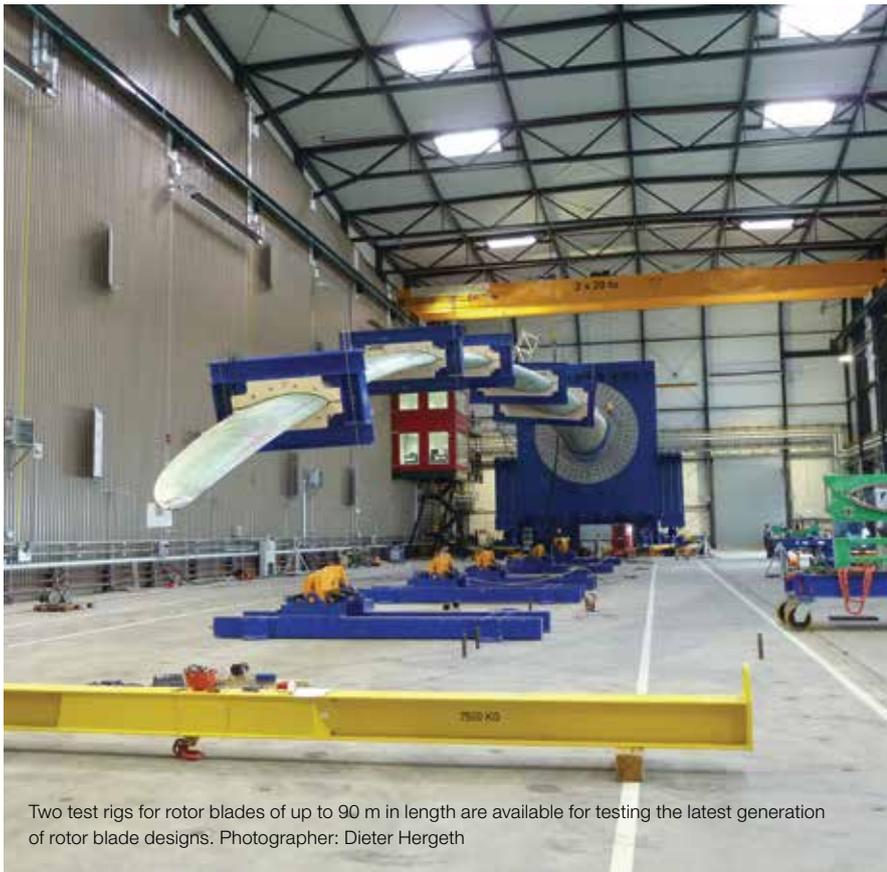
Two test rigs for rotor blades of up to 90 m in length are available for testing the latest generation of rotor blade designs. Photographer: Dieter Hergeth
