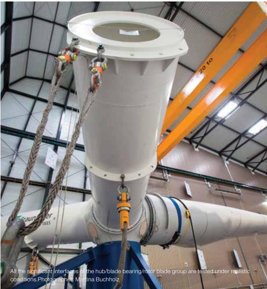
All the significant interfaces of the hub/blade bearing/rotor blade group are tested under realistic conditions. Photographer: Martina Buchholz
