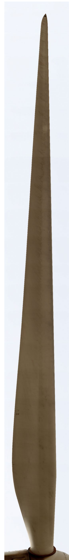
Mosaic automatically composed from 25 different images of the blade
