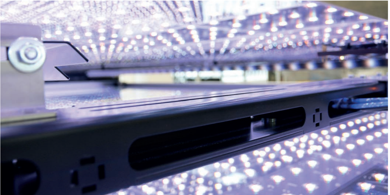
Figure 2: LED sun simulator with two LED units for the measurement of bifacial modules
